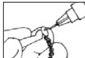
3. Extrude Adhesive over previously applied Activator on back of mesh pad and immediately place attachment.
