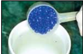
2. Drop 1/2 scoop of Aquaform into less than boiling water (180°F) for 20 seconds. Remove, then knead with fingers until the color is even.
